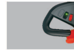
Four colored LED battery meter
