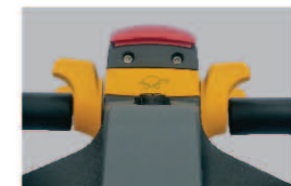
The turtle speed switch on the handle makes low speed control more precise.
