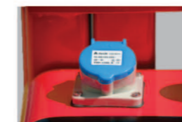
Air Plug Connects Battery And Charger
