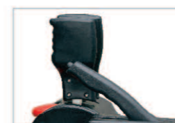
Hand brake and handle is set on the right side, which meets the ergonomic principles. It reduces the operator's labor intensity and improves the operation comfort.
