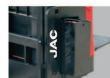
Side-pull feature for batteries is optional.
